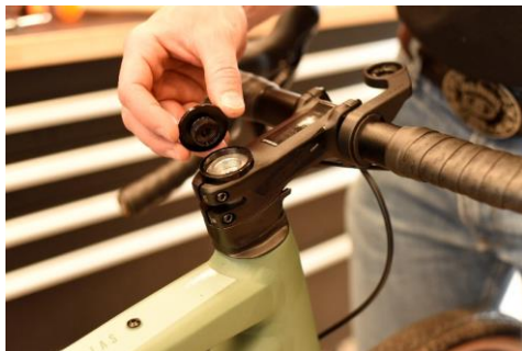
24. Put the required spacer on the top. Then, assemble the headset compressor
