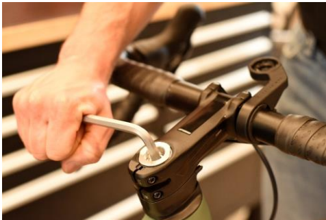
5. Release the expander using an 8 mm Allen key
