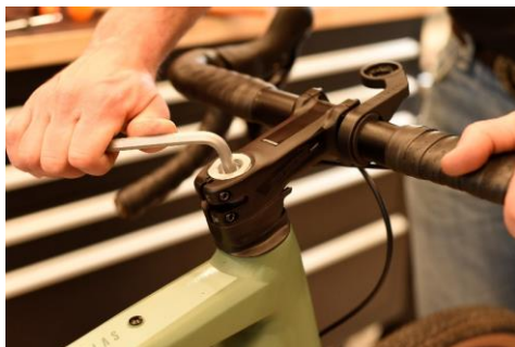
22. Using an 8 mm Allen key, tighten the expander at 15Nm
