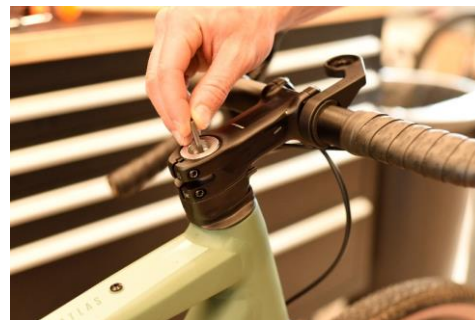
23. Insert the lockout shaft, be sure to engage the seat correctly
