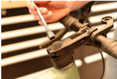
7. Add grease to the 13mm socket wrench so that the top cap nut will stick to the socket once loosened.
