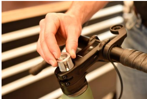
6. Remove the expander by hand
