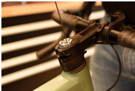
13. Pull out the top cap using a pick.
