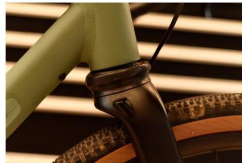
11. The suspension will easily compress once the top cap has been loosened
