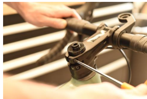
26. Tighten the stem screws according to the component's specs.
