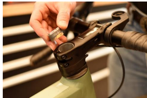
16. Insert the top cap in the steerer
