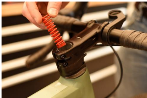
16. Make sure the preload spacer is downwards and the spring upwards
