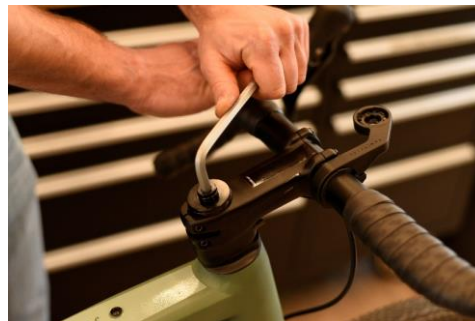
3. Remove the headset compressor using an 8mm Allen key
