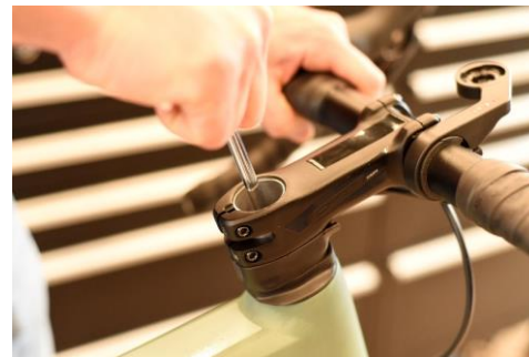
8. Unscrew the top nut in the steerer.
