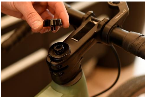
1. Remove the lock-out knob
