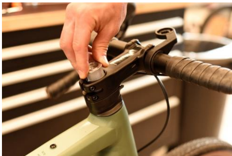
21. Insert the expander in the steerer by hand
