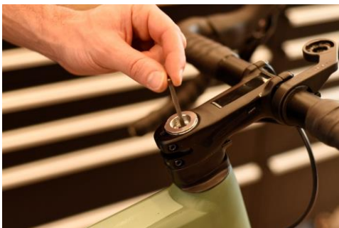
4. Remove the lock-out shaft
