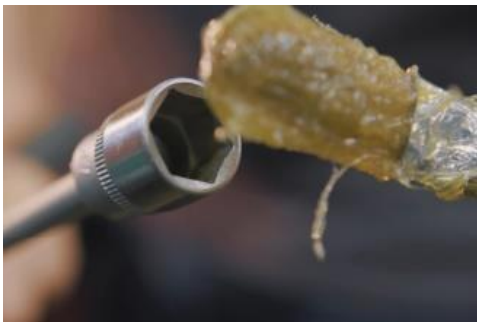
7. Add grease to the 13mm socket wrench so that the top cap nut will stick to the socket once loosened.
