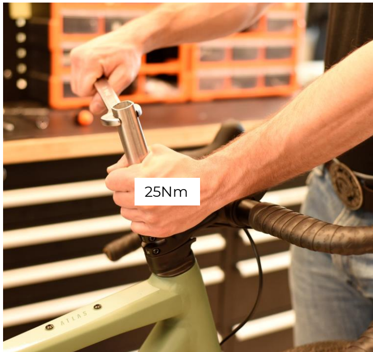
17. Tighten the top cap to 25 Nm using the 24mm wrench while keeping the suspension extended
