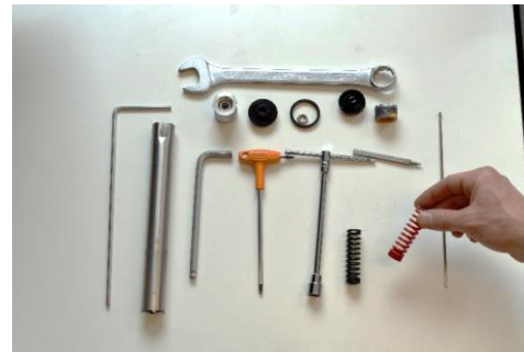
15. Select a new spring and preload (information provided in the last pages)
